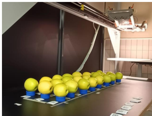
Figure 1. Set-up of hyperspectral cameras to image apples in horizontal position with their corresponding QR codes.
