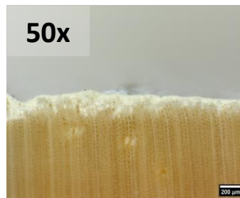
Figure 1. Example of a microscope image for individual assessment of coating thickness.
