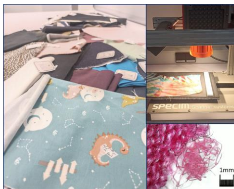
Figure 1. Some textile samples, example of acquisition process, and image of sample with elastane
