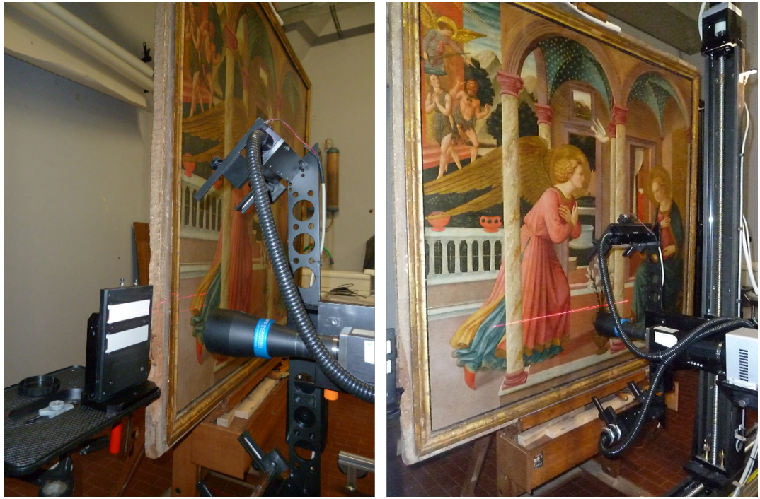
Fig. 1. Reflectance Hyperspectral Imaging IFAC-CNR Scanner. Measurements on a Renaissance painting (1450 ca) from the Florentine School of Beato Angelico. Soprintendenza Labs, Uffizi Gallery (Firenze).
